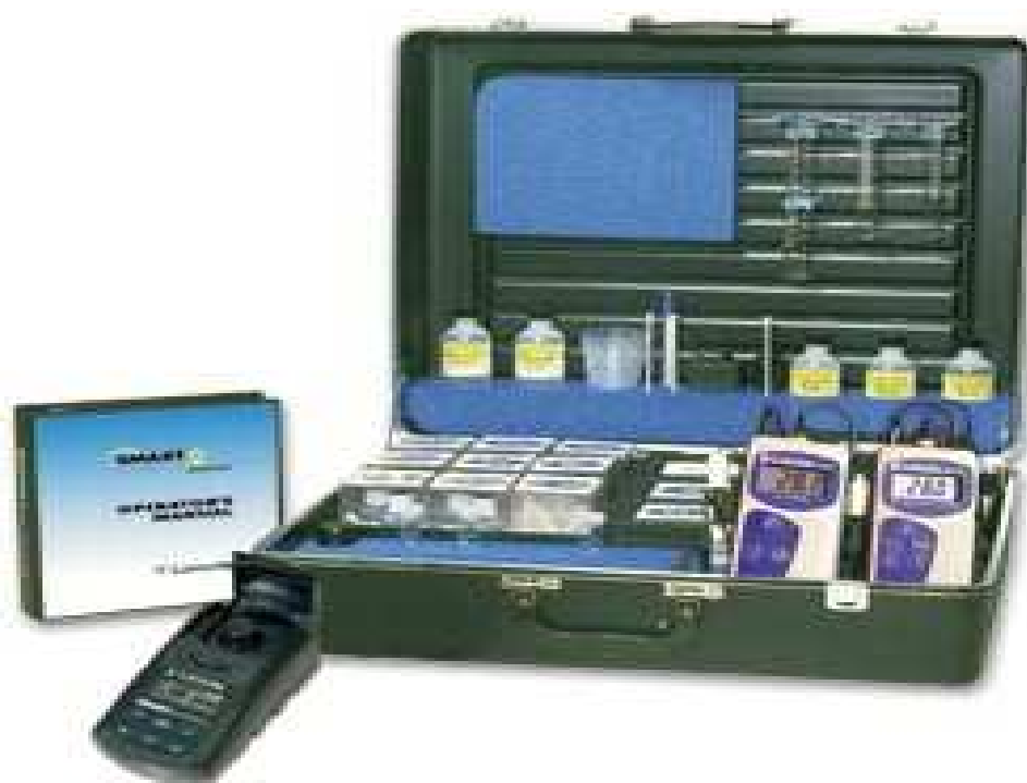
Figura 7 Kit de campo Smart Water Análisis Laboratory.
