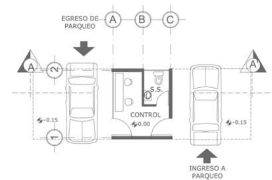
GARITA DE CONTROL VEHICULAR
