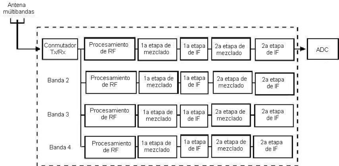
Figura 4 Arquitectura tradicional de múltiples bandas; adaptación de la figura 12 “Super heterodyne architecture with two stages for traditional multi-bands receiver” del documento 11 de OverDRIVE *
