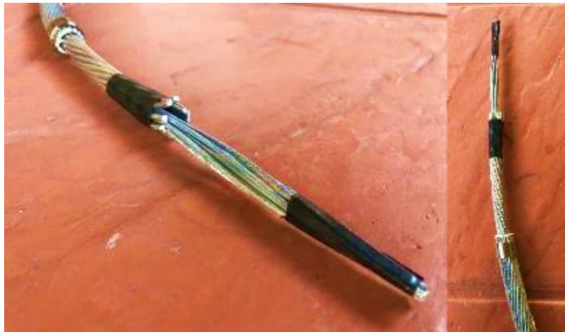
Figura 25. Cable aluminio sin forro 477,0 ACSR (hawk)
