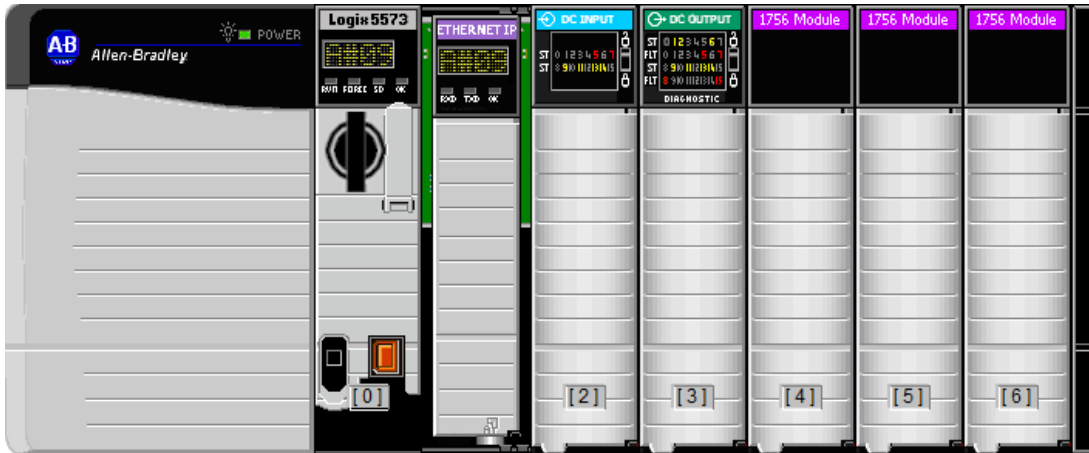
Figura 5. PLC Allen Bradley ControlLogix 1756 L73
