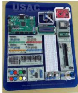
Fig. 1. Prototype: modular educational board
