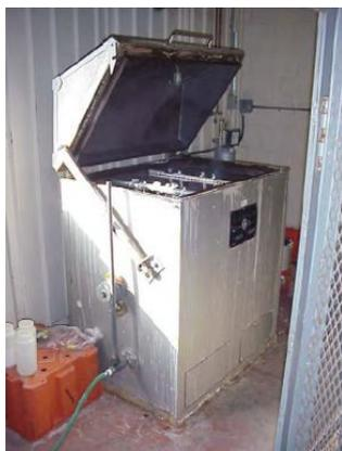
Fuente: COLBERT, M. Salt spray corrosion test on 1 020 kcmil ACCC/TW conductor. p. 5.
