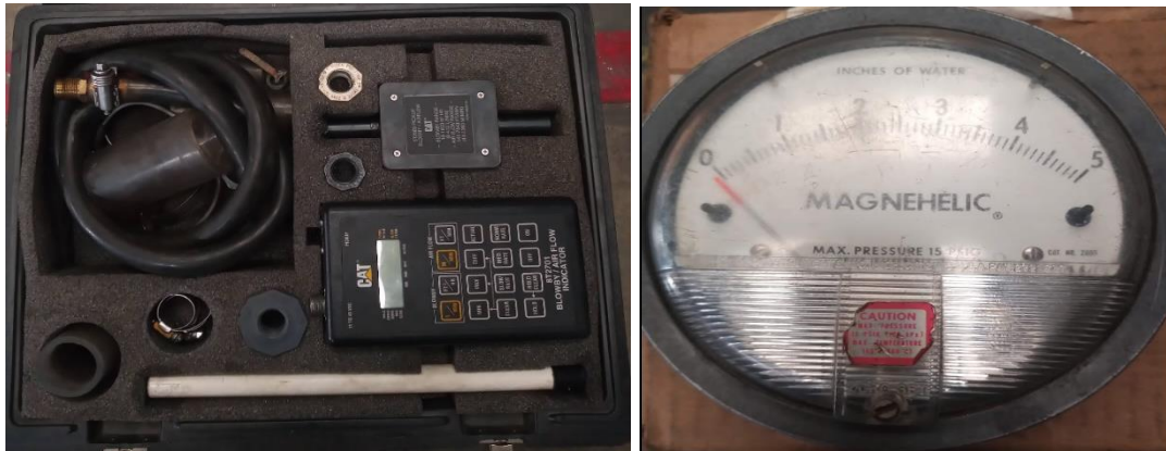
Figura 15. Caterpillar blowby group 8T2700 y magnehelic
