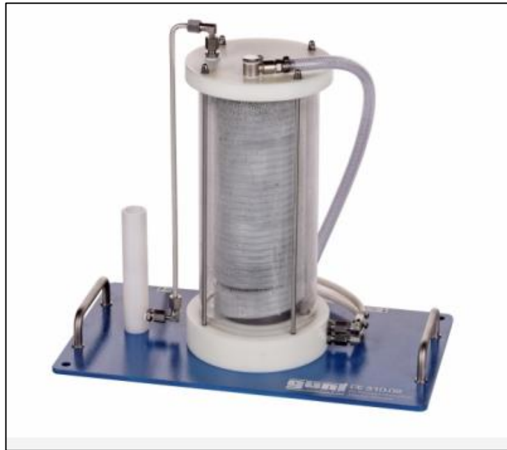
Figura 18. Reactor PFR Helicoidal
