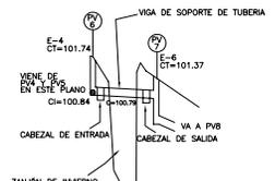
DETALLE DE PASO AÉREO ENTRE PV6 Y PV7 - PV14 Y PV15
