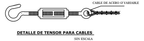
**DETALLE DE TENSOR PARA CABLES**
