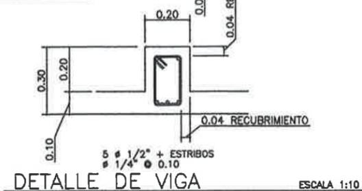
DETALLE DE VIGA ESCALA 1:10
