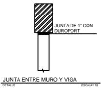
JUNTA ENTRE MURO Y VIGA
